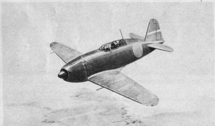
Jack 11 is a fat stubby 400-mph. fighter, somewhat resembling the earlier Tojo. Three-view silhouette of Jack will be found on page 17.
